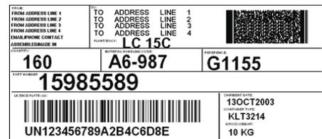
Error Proof® also contains a sophisticated WIP label to track work-in-process. The WIP label can be produced at the part or at the container level, thus providing a tracking mechanism throughout the production process. This label is unique in that it combines the bill and router with the label to be used for additional error proofing processes.
