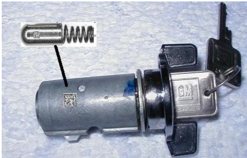
Ignition switch with serialized 2D code could have prevented widespread recall
